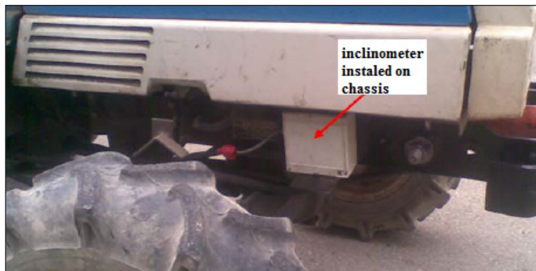
Figure 6. Inclinometer installed on chassis
